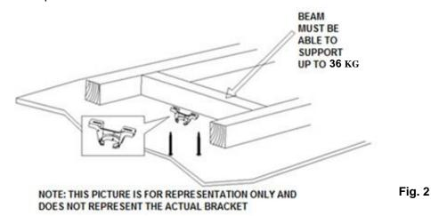
NOTE: The bracket screws provided are for use with wooden structures only. For structures other than wood, the appropriate screw type MUST be used. Ensure the screws used are suitable for the mounting surface and the surrounding environment.
