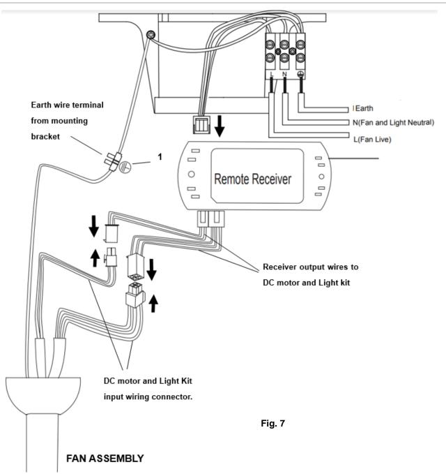
Carefully insert the Remote Receiver above the hanger ball in the remainder spacing in the mounting bracket. Take care not to damage or loosen any of the wiring. (Fig. 8).
