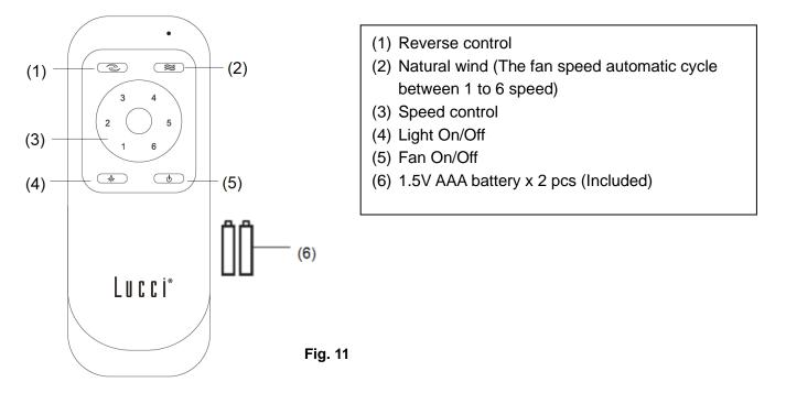
The LED globe has a 3-step dimmable function which is controlled by an ON/OFF switch. When the LED light is ON and at 100% brightness, press the light button "ON and then OFF within 3 seconds", to dim the LED light. Repeat pressing ON and then OFF within 3 seconds to dim further in the following sequence: 100% brightness  $\rightarrow$  50% brightness  $\rightarrow$  15% brightness  $\rightarrow$  100% brightness.
